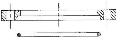
Rotatable Bolt Ring converts an ISO-K to an ISO-F Bolt type flange. For dimensions, please ask for data sheet.
