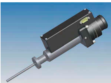
Drive with limit switch box. A single Sub-D connector is used for stepper motor connection and mechanical limit switches
