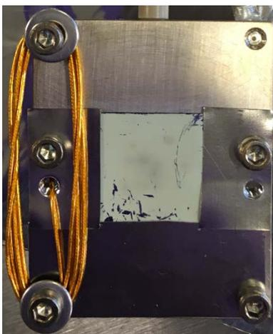
Figure 1: Image of the 301-KAPM-060 wire sample mounted on the electron-beam chamber sample holder.
